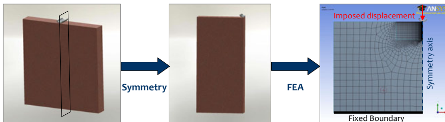
Fig. 3: Highlight of the simplification process to obtain the 2D model
